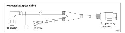
The array and the display should be connected using the pedestal adaptor cable as shown:
